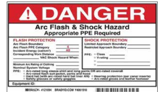
Figure 2. Arc Flash & Shock Hazard Warning
