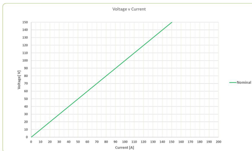
Figure 10.1: NGR Current/Voltage Graph
